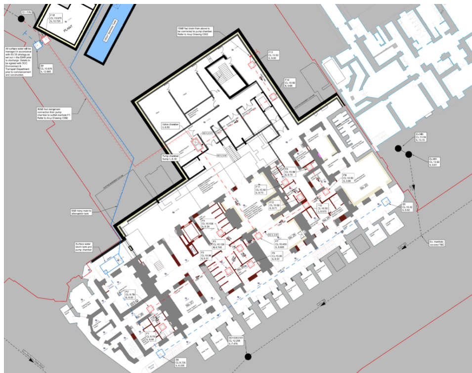
Figure 5.9.7: Foul Drainage- Proposed
