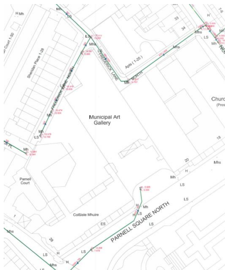
Figure 5.9.2: Combined Sewers - Existing
